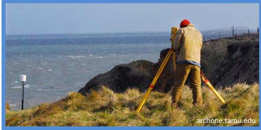
short distances, within the order of a few millimetres. However, along the coast, where humidity is omnipresent and the atmospheric distortions are common, measurement quality deteriorates quickly. Distance of the unit relative to the prism is also a limiting factor that causes measurement quality to decrease. During a coastal study in northern New Brunswick, it was found that distances between the
