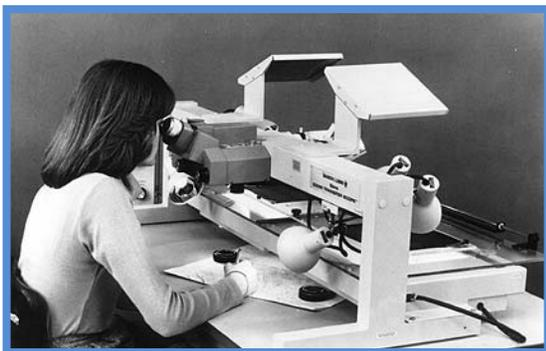
matching of a variety of sources (such as aerial photos, plates, and surveys) to a base map (such as a topographic map or a bathymetric map): it displays two images superimposed on a single display at nearly the same scale and orientation. Once the zoom lens is adjusted for scale differences, data can be transferred (or traced) manually to a base overlay, such as a mylar or acetate. The procedure requires that the base document (for example a topographic map) be
