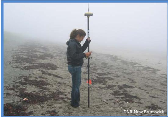
in the static mode, i.e. when the measure is made on one point during many consecutive minutes or even hours. When the unit is set in the roaming or kinematic mode (RTK) – many readings registered in a short time along a path or transect, as is typically the case – the accuracy tends to fall, but generally remains under 5 cm. In fact, many *GPS-RTK* units are set to accept readings that are no greater than a maximum of 5 cm horizontally (x,y) and no greater than 10 cm vertically (z).
