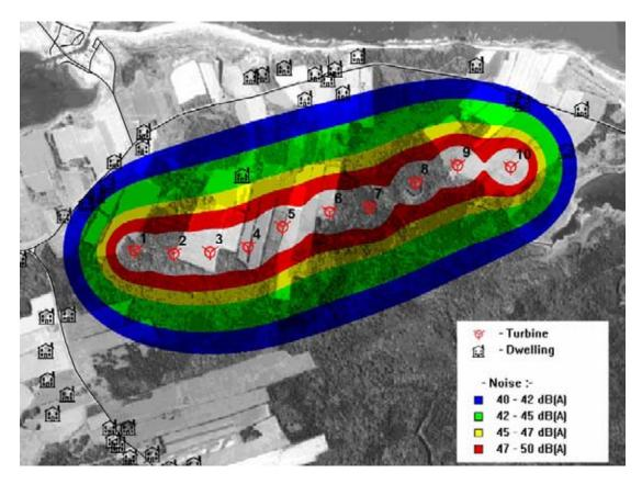
Figure 5.1. Predicted noise level contours resulting from wind plant operation
