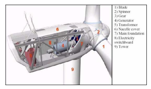
Figure 3.2. Components of the V90 nacelle (Vestas, 2005)
