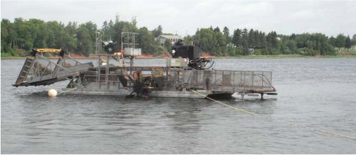
Figure 1. Aquarius 170 aquatic harvester used in project.
