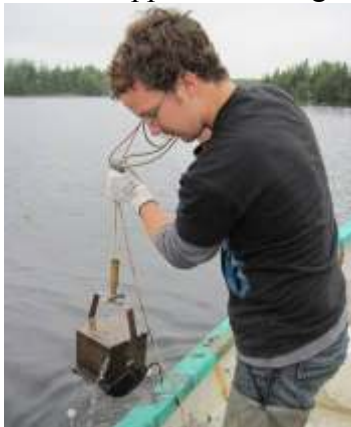
Figure 15. Sampling bottom sediments with Ekman grab.
