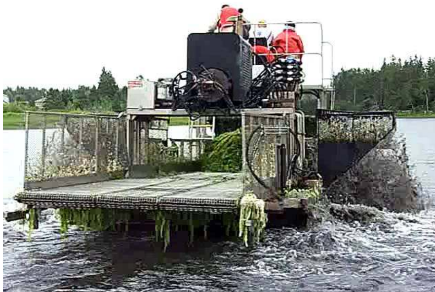
Figure 16. Sediments disturbed by paddle wheels.
