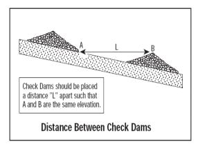
Check dams are temporary structures made from stones, straw bales, sandbags, or logs constructed across a ditch to reduce the velocity of the concentrated flow and thereby the potential for erosion until permanent stabilization of the disturbed area has been established.
