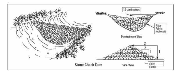
elevation of the toe of the upstream dam is the same elevation as the top of the downstream dam.
