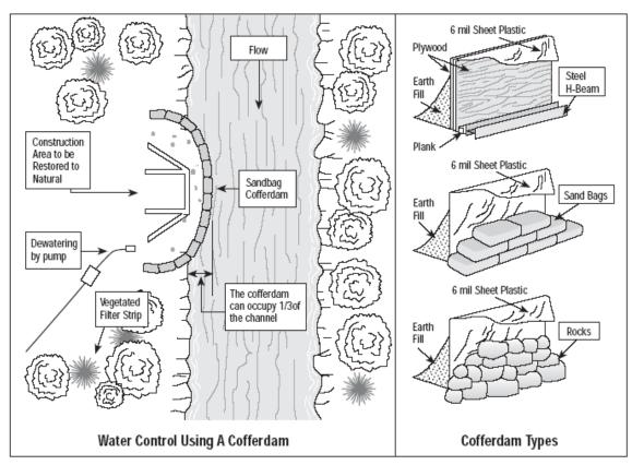
**Cofferdams** can be constructed to isolate the work area from flowing water. At least two-thirds of the cross-sectional area of the channel must be open at all times. Cofferdams may consist of: sheet piling or a layer of 6 mil plastic sandwiched between an inner wall of in situ earth fill and an outer
